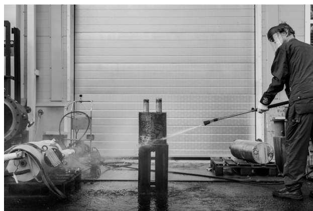
High-pressure water cleaning of a plate pack at Vahterus manufacturing facilities in Kalanti, Finland.
